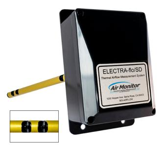
Multiple pairs of surface mounted precision thermistors utilize the principle of thermal dispersion to accurately measure both average flow velocity and air temperature within the duct.
